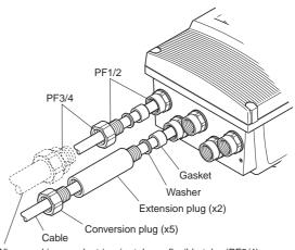
When working on electric wire tube or flexible tube (PF3/4) \* When connecting PF1/2, remove the conversion plug and connect directly to wiring port.
